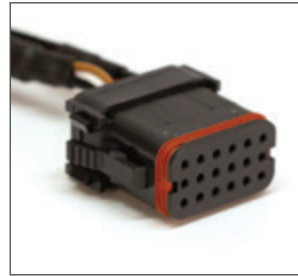
E050 Configuration Harness (Part No. 016-177) Coded AMP SEAL connector configuration harness pre-wired with 0.5 metre (1 ft 7") CAN cable and 1.0 metre (3 ft 3") DC power cable
